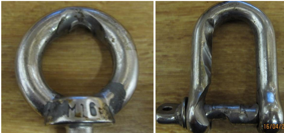
Figure A1 Excessive wear to an eyebolt and shackle due to vibrations caused by cavitation.
